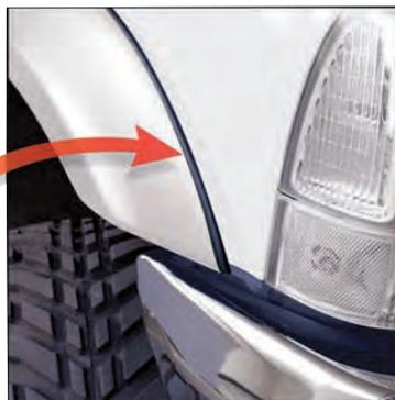
Easily installed before fender flare is installed against body to isolate vibration and provide an attractive finish.
